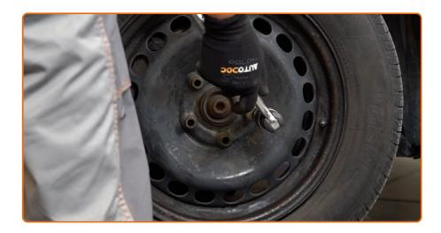
Lower the car and working in a cross order, tighten the wheel bolts. Use wheel impact socket #21. Use a torque wrench. Tighten it to 120 Nm torque.
