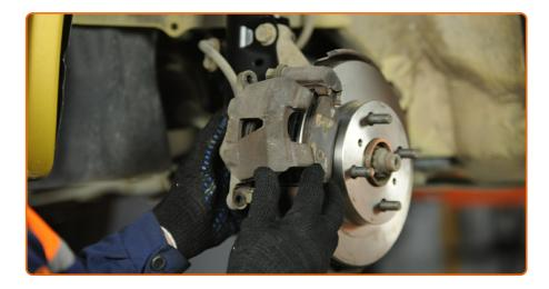
Remove the brake caliper.
