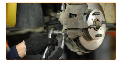
Install the brake caliper and fix it. Use a combination spanner #17. Use a drive socket #14. Use a torque wrench. Tighten it to 35 Nm torque.
