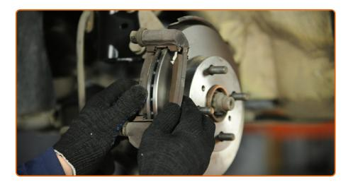
Remove the brake pads.
