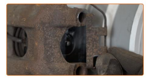
Install the brake caliper retaining spring.
