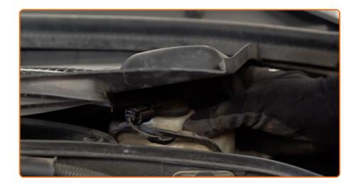
Tighten the brake fluid reservoir cap.
