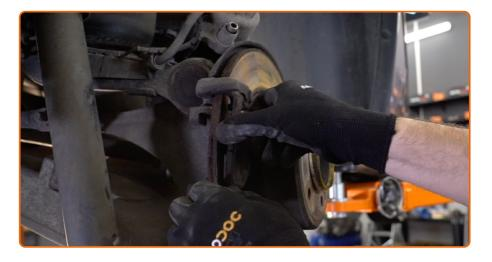
Remove the brake pads. Use a crowbar.
