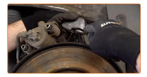
Remove the connector of the brake pad wear sensor. Use a crowbar.
