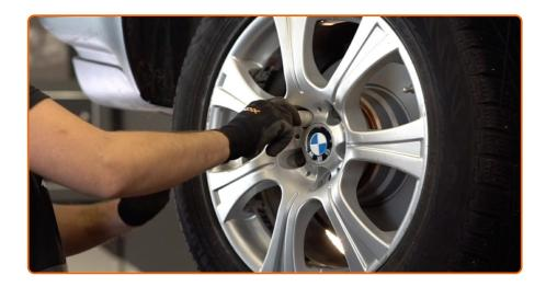
Screw in the wheel bolts. Use wheel impact socket #19.
