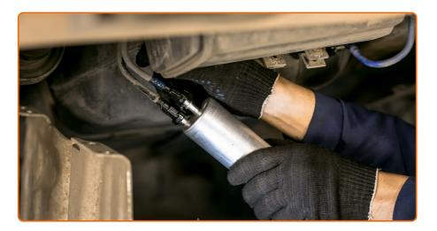
Attach the tubes to the fuel filter.
