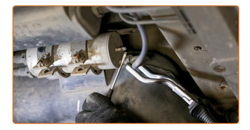
Detach the tubes from the fuel filter. Use a flat screwdriver. Use fuel line pliers.
