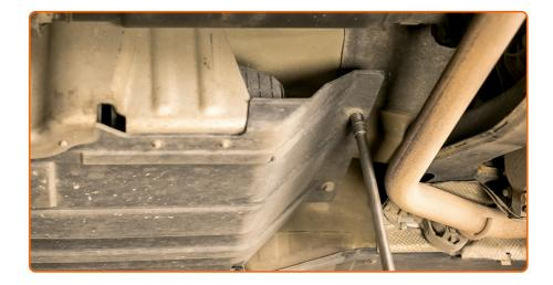
Unscrew and remove the oil pan cover.
