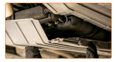
Install the oil pan cover and screw in its fasteners.
