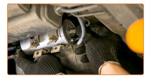
Attach the tubes to the fuel filter.
