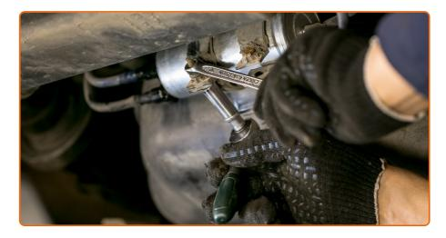
Screw in the fuel filter mounting bracket. Use a combination spanner #10. Use a drive socket #10. Use a ratchet wrench.
