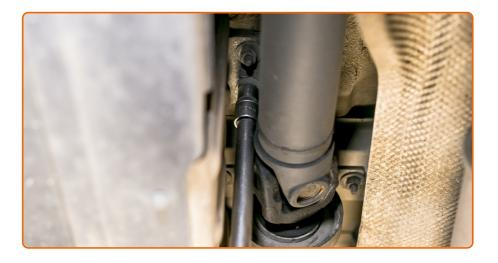
Unscrew the fasteners of the propeller shaft centre support bearing. Use a drive socket #13. Use a ratchet wrench.
