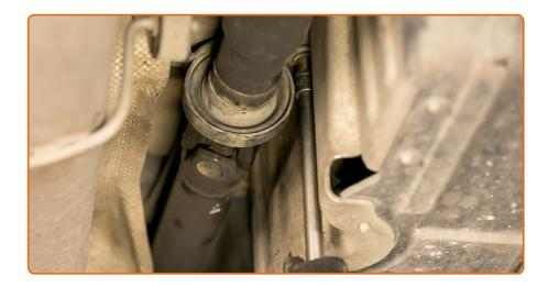
Tighten the fasteners of the propeller shaft centre support bearing. Use a drive socket #13. Use a torque wrench. Tighten it to 55 nm torque.
