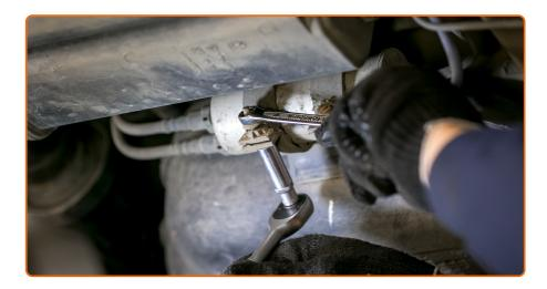
Loosen the fuel filter mounting. Use a combination spanner #10. Use a drive socket #10. Use a ratchet wrench.
