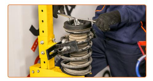
Tighten the shock strut piston rod nut. Use a combination spanner #21. Use HEX No.H7. Use a torque wrench. Tighten it to 60 Nm torque.
