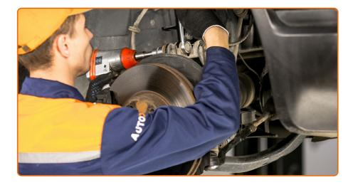
Tighten the lower fasteners connecting the shock strut to the steering knuckle. Use a combination spanner #22. Use a drive socket #22. Use a torque wrench. Tighten it to 75 Nm torque.
