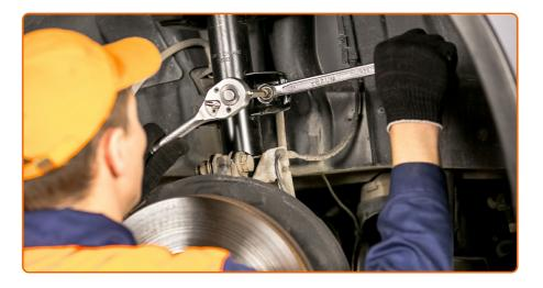
Tighten the fastener connecting the stabilizer link to the shock strut. Use a combination spanner #19. Use HEX No.H5. Use a torque wrench. Tighten it to 55 Nm torque.
