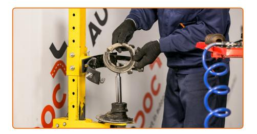
Remove the rubber spring spacer.
