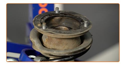
Install the upper strut mount and the strut mount bearing.
