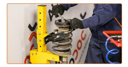
Remove the strut piston rod nut. Use a combination spanner #21. Use HEX No.H7.
