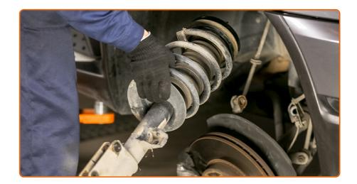
Remove the suspension strut.
