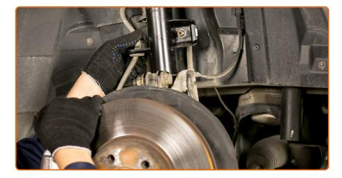
Fasten the brake hose on the strut.
