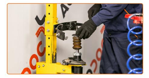
Install the dust sleeve and the bump stop on the new shock absorber.
