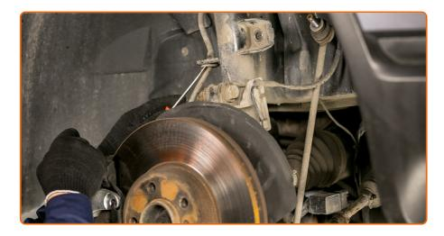
Detach the brake hose from the shock strut. Use a flat screwdriver.
