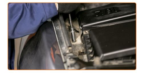
Unscrew the bolts and remove the windshield washer tank. Use a drive socket #10. Use a ratchet wrench.
