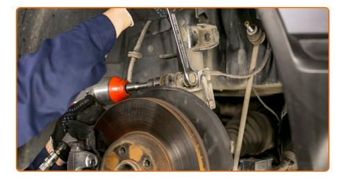
Unscrew the lower fastener connecting the shock strut to the steering knuckle. Use a combination spanner #22. Use a drive socket #22. Use a ratchet wrench.
