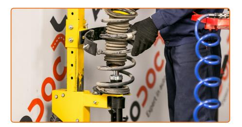
Install the spring on the shock absorber.
