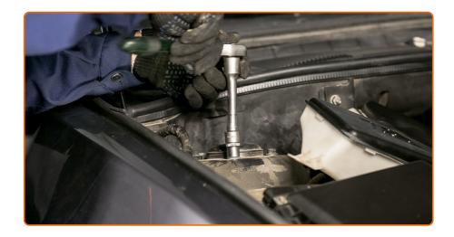
Tighten the upper fastener of the shock absorber strut mount. Use a drive socket #13. Use a torque wrench. Tighten it to 37 Nm torque.
