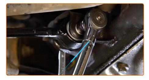
Tighten the arm fastening to the subframe. Use a drive socket #18. Use a combination spanner #18. Use a torque wrench. Tighten it to 90 nm torque.
