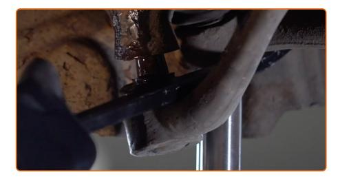
Remove the ball joint from the steering knuckle. Use a crowbar.
