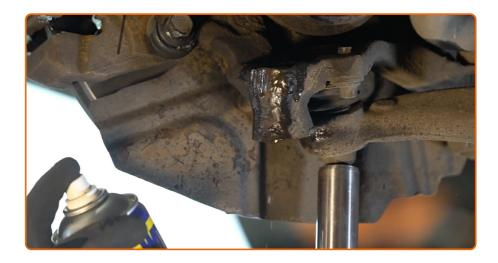
Clean the mounting seats and the thread of the suspension arm.
