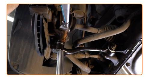
Tighten the ball joint fastening nut. Use a combination spanner #22. Use a torque wrench. Tighten it to 80 nm torque.
