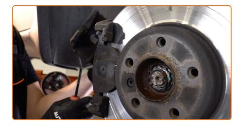
Remove the brake caliper.
