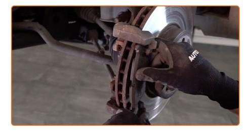
Remove the brake pads. Use a crowbar.
