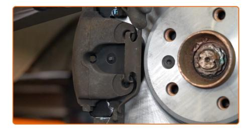
Install the brake caliper retaining spring.
