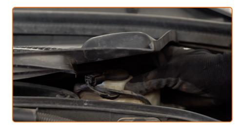
Tighten the brake fluid reservoir cap.
