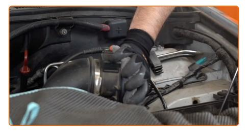
Before cleaning the air filter cover and housing, cover the air duct parts, mass airflow sensor (if available), throttle valve with a clean cloth.
