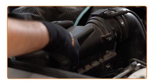
Reinstall the air filter cover. Fasten it.
