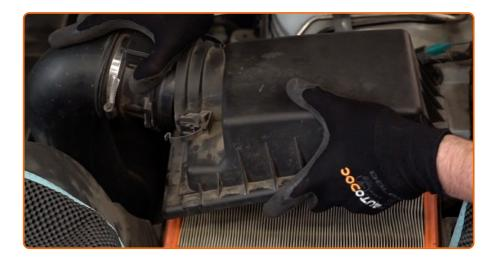
Disconnect the air intake pipe from the air filter housing.
