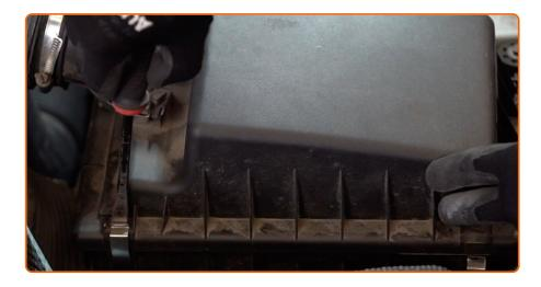
Release the air filter cover clips. Use a crowbar.
