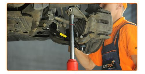
Fix the shock absorber strut on the steering knuckle. Use a hammer.
