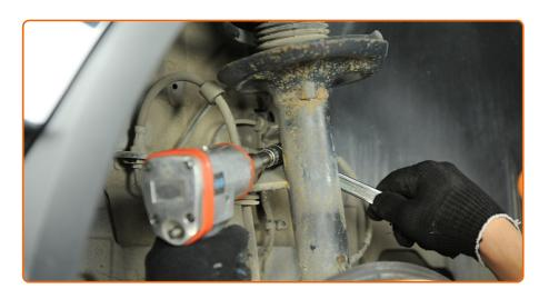
Unscrew the fastener connecting the stabilizer link to the shock strut. Use a combination spanner #19. Use a drive socket #16. Use a ratchet wrench.
