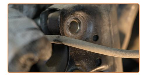
Remove the fastening bolt.
