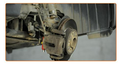
Disconnect the steering knuckle from the shock absorber strut. Use a hammer.
