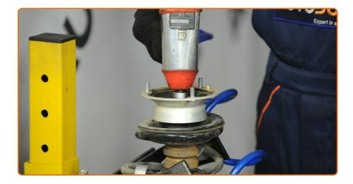
Remove the strut piston rod nut. Use a drive socket #22. Use a ratchet wrench.
