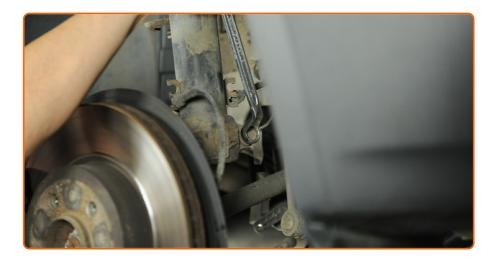
Unscrew the lower fastener connecting the shock strut to the steering knuckle. Use a combination spanner #16. Use a drive socket #18. Use a ratchet wrench.
