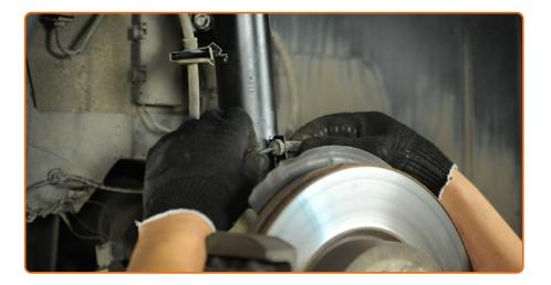
Connect the ABS sensor wiring.
