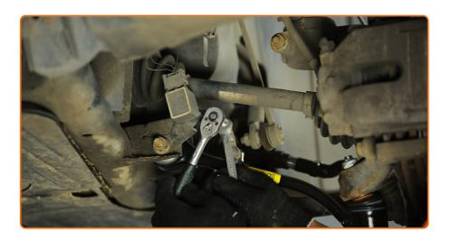
Unscrew the fasteners of the headlight levelling sensor. Use a combination spanner #10. Use a drive socket #10. Use a ratchet wrench.
