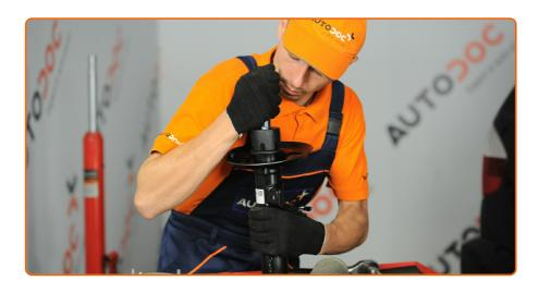
Install the new shock absorber on the hydraulic coil spring compressor.
