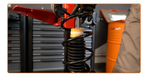
Install the spring on the shock absorber.
