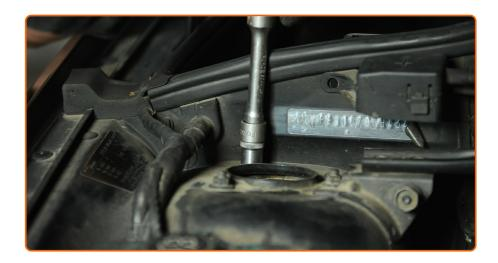
Unscrew the top fastening of the shock strut mount. Use a drive socket #13. Use a ratchet wrench.
