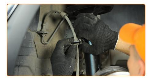
Fasten the brake hose on the strut.
