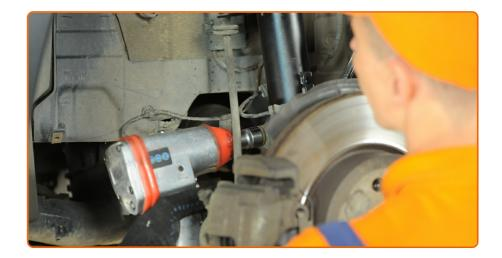
Tighten the lower fasteners connecting the shock strut to the steering knuckle. Use a combination spanner #16. Use a drive socket #18. Use a torque wrench. Tighten it to 80 Nm torque.
