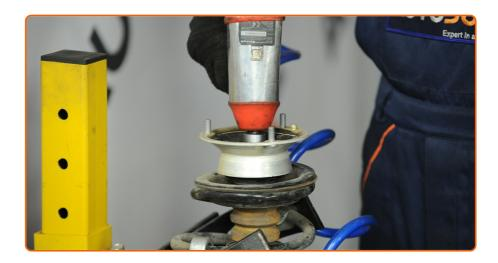
Tighten the shock strut piston rod nut. Use a drive socket #22. Use a torque wrench. Tighten it to 65 Nm torque.
