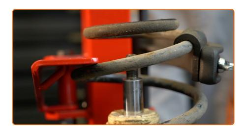
Release the coil spring.
