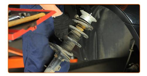
Remove the suspension strut.
