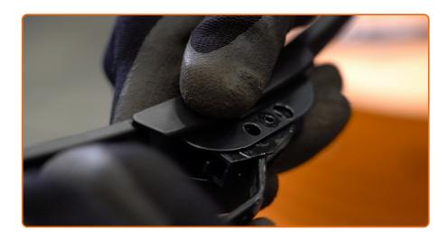
Install the new wiper blade and carefully press the wiper arm down to the glass.
