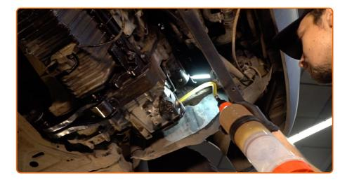
Pour the oil into the gearbox through the filler hole. Required amount of oil: 2.5 L.
