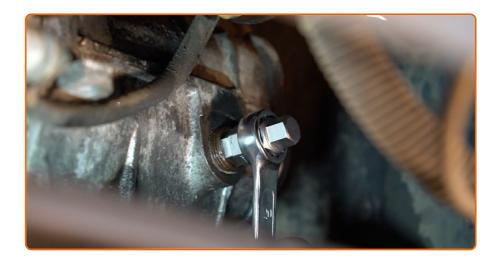
Unscrew the filler plug of the gearbox housing. Use HEX No.H17.
