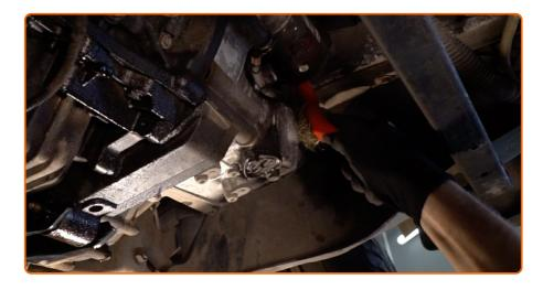
Clean the area around the gearbox housing filler hole.
