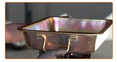
Put a waste oil container with at least 3 I capacity under the drainage hole.
