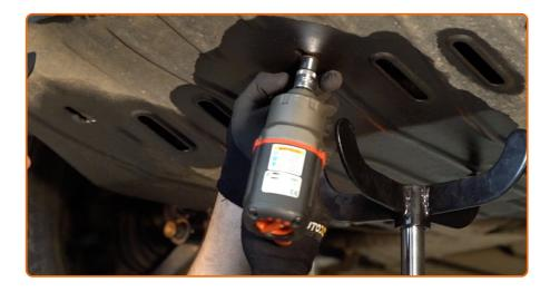
Undo the fasteners of the oil pan lower cover. Use a drive socket #12. Use a Phillips screwdriver.
