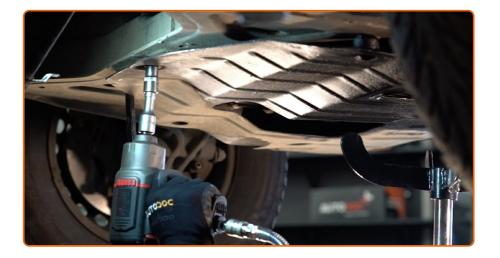
Tighten the fasteners of the oil pan lower cover. Use a drive socket #12. Use a Phillips screwdriver. Lower the car.
