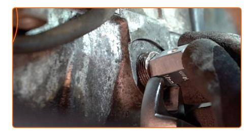
Screw in the filler plug of the gearbox housing. Use HEX No.H17. Use a torque wrench. Tighten it to 29 Nm torque.
