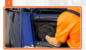
Disconnect the mounting of the pipe supplying air into the cabin.
