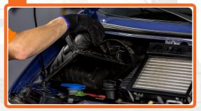
Reinstall the air filter cover. Fasten it.
