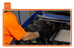
Install the air supply pipe and fasten it.
