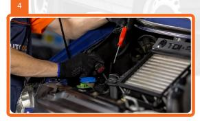
Disconnect the wiring from the mass air flow sensor.
