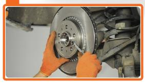
Tighten the brake disc fastening
