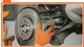
Install the brake caliper and fix it.
