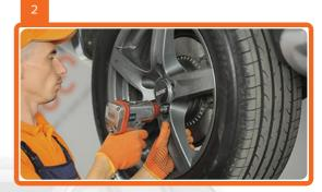
Loosen the wheel mounting bolts.
