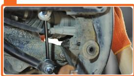
Unscrew the wheel hub axle nut.
