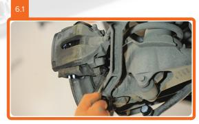
Unscrew the brake caliper fastening
