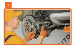
Remove the brake caliper.
