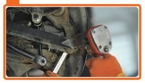
Unscrew the rear transverse arm fastener to the stub axle.
