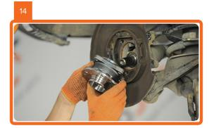
Install the wheel hub on the steering knuckle.
