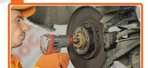
Loosen and remove the hub nut.
