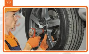
Lower the car and working in a cross order, tighten the wheel bolts.
