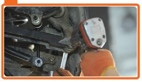
Tighten the control arm fastener to the stub axle.
