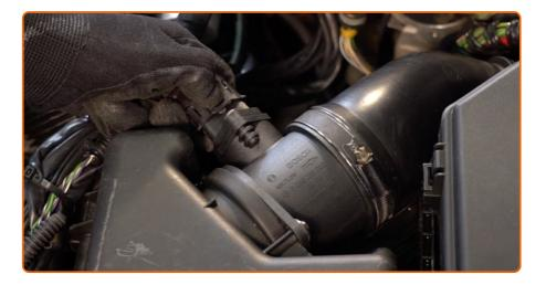
Unplug the mass air flow sensor connector.
