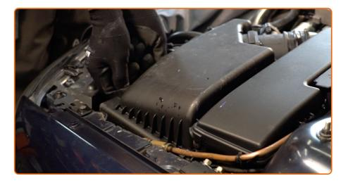
Release the air filter cover clips.
