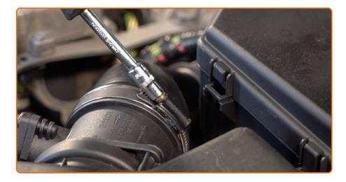
Detach the air intake hose clamp. Use a drive socket #7. Use a ratchet wrench.
