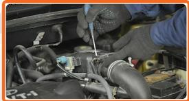
Disconnect the wiring from the mass air flow sensor.
