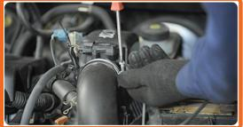
Secure the inlet air hose on the filter housing with a clamp.
