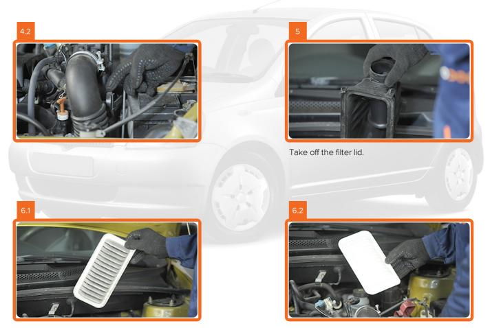
Remove the air filter and replace it with a new one.
