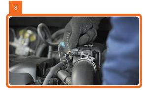
Connect the wiring to the mass air flow sensor.
