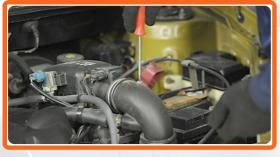
Loosen the clamp and remove the intake air hose from the filter housing.
