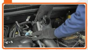
Reinstall the air filter cover. Fasten it.
