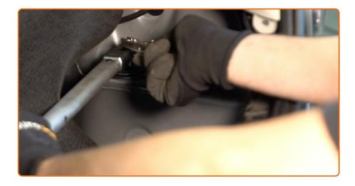
Tighten the top shock absorber fastening. Use a combination spanner #14 (2 pieces). Use locking pliers. Use a torque wrench. Tighten it to 65 Nm torque.
