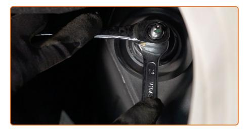
Unscrew the upper fastener of the shock absorber. Use a combination spanner #14 (2 pieces). Use locking pliers.
