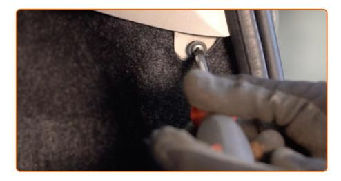
Unscrew the fastener of the boot side lining. Use a Phillips screwdriver.
