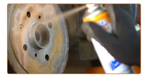
Treat the contacting surface. Use copper grease.
