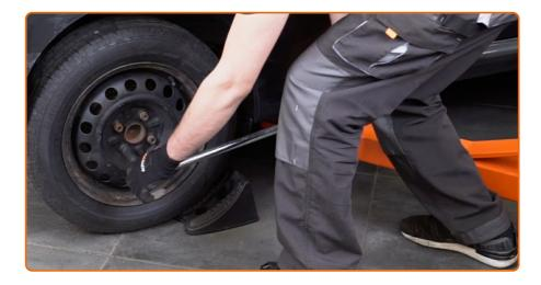
Tighten the wheel bolts using a criss-cross pattern. Use a torque wrench. Tighten it to 120 nm torque.
