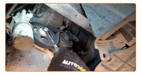
Tighten the tensioner lever of the V-ribbed belt. Use a combination spanner #12. Use a drive socket #14. Use a ratchet wrench.
