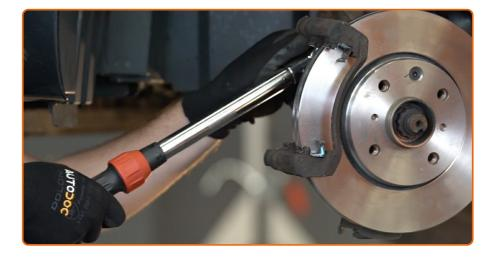
Tighten the brake caliper bracket. Use a drive socket #17. Use a torque wrench. Tighten it to 65 Nm torque.
