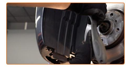
Unscrew the brake disc fastening. Use a Phillips screwdriver.
