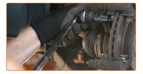
Unscrew the caliper bracket fastening. Use a drive socket #17. Use a tap wrench. Use a ratchet wrench.
