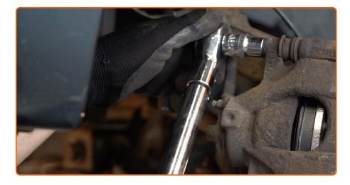
Install the brake caliper and fix it. Use a drive socket #13. Use a torque wrench. Tighten it to 35 Nm torque.
