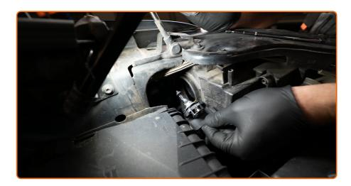
Install a new bulb into the holder.
