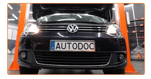
Switch on the headlights to check whether the new lamp functions properly.
