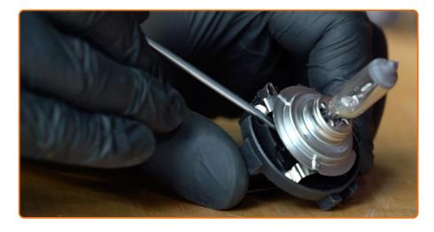
Remove the old bulb. Use a flat screwdriver. Check the condition of the bulb holder terminals. Replace if necessary.
