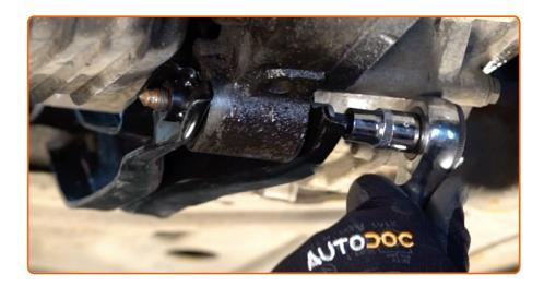
Tighten the fastening bolt connecting the engine mount to the gearbox housing. Use HEX No.H10. Use a torque wrench. Tighten it to 57 Nm torque.
