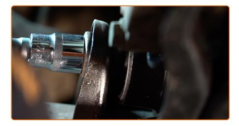
Screw in the engine mount fasteners. Use HEX No.H10. Use a drive socket #21. Use a ratchet wrench.
