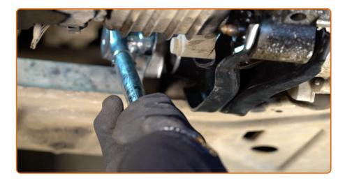
Tighten the fastening bolt connecting the engine mount to the subframe. Use a drive socket #21. Use a torque wrench. Tighten it to 65 Nm torque.
