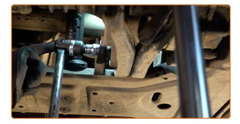
Unscrew the engine mount fastener that connects it to the subframe. Use a drive socket #21. Use a ratchet wrench.
