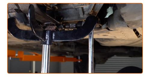
Unscrew the fastener connecting the engine mount to the gearbox housing. Use HEX No.H10. Use a ratchet wrench.
