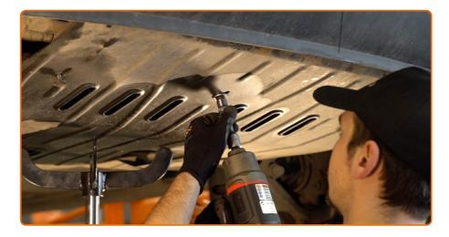
Tighten the fasteners of the oil pan lower cover. Use a drive socket #12. Use a Phillips screwdriver.
