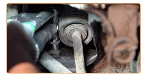
Screw the fasteners of the stabilizer bush brackets. Use a drive socket #16. Use a torque wrench. Tighten it to 45 nm torque.
