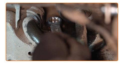
Unscrew the fasteners of the stabilizer bush brackets. Use a combination spanner #16. Use a drive socket #16. Use a ratchet wrench.
