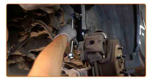
Install a new rod, tighten the fasteners. Use a drive socket #17. Use a ratchet wrench.
