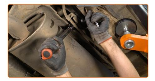
Tighten the fastener connecting the control arm to the car body. Use a combination spanner #17. Use a drive socket #17. Use a torque wrench. Tighten it to 75 nm torque.
