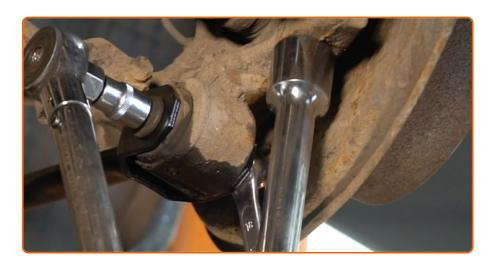
Tighten the fastener connecting the suspension arm to the rear knuckle. Use a combination spanner #18. Use a drive socket #E18. Use a torque wrench. Tighten it to 80 nm torque.
