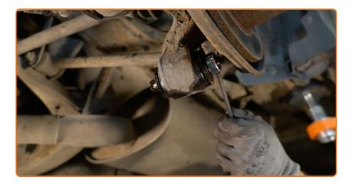
Loosen the fastener that connects the control arm to the rear knuckle. Use a combination spanner #18. Use a drive socket #E18. Use a tap wrench.
