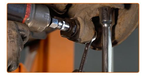
Unscrew the fastener connecting the control arm to the rear knuckle. Use a combination spanner #18. Use a drive socket #E18. Use a tap wrench.
