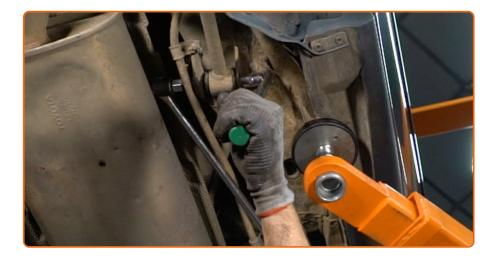
Unscrew the fastener connecting the trailing arm to the car body. Use a combination spanner #17. Use a drive socket #17. Use a tap wrench.
