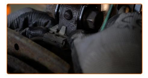
Connect the fastener of the ABS sensor cable to the shock absorber strut.
