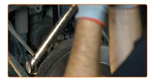
Tighten the lower fasteners connecting the shock strut to the steering knuckle. Use a drive socket #21. Use a torque wrench. Tighten it to 90 Nm torque.
