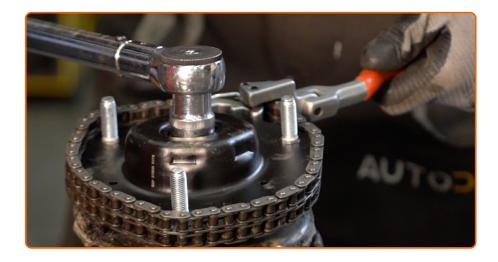
Tighten the shock strut piston rod nut. Use a drive socket #21. Use a chain wrench. Use a torque wrench. Tighten it to 60 Nm torque.
