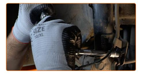
Disconnect the brake hose holder from the shock absorber strut. Unscrew the ABS sensor fastener. Use a drive socket #12. Use a ratchet wrench.
