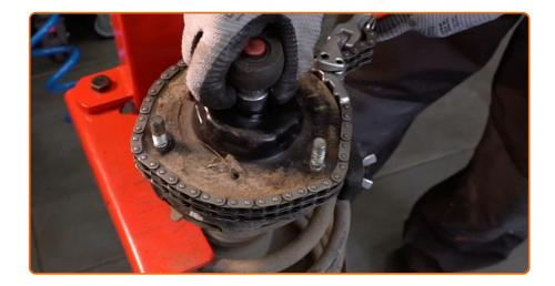
Remove the strut piston rod nut. Use a chain wrench. Use a drive socket #19. Use a ratchet wrench.
