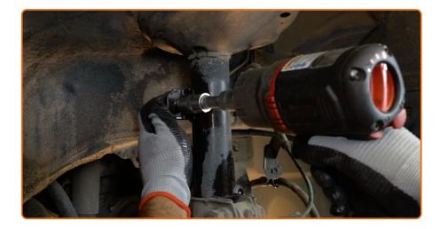
Unscrew the fastener connecting the stabilizer link to the shock strut. Use a drive socket #17. Use a ratchet wrench.
