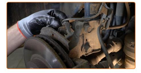
Detach the fastener connecting the ABS sensor cable to the shock strut.
