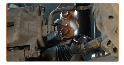
Treat the shock strut fasteners. Use copper grease.
