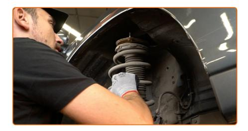
Remove the suspension strut.
