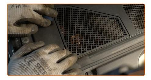
Install the suspesion strut mount cap.
