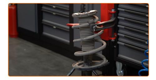
Release the coil spring.
