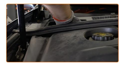
Screw the top fastening of the shock strut mount. Do not tighten it.
