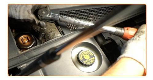
Tighten the upper fastener of the shock absorber strut mount. Use a drive socket #14. Use a torque wrench. Tighten it to 50 Nm torque.
