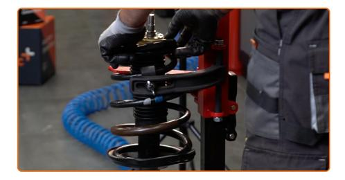
Install the mount, the boot and the bump stop on the shock absorber.
