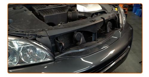
Remove the fender protection cover.
