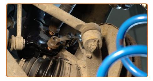
Screw in the fastener that connects the shock strut to the steering knuckle. Use a combination spanner #21. Use a drive socket #21.
