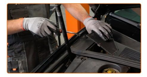
Remove the suspension strut mount cap. Use a crowbar.
