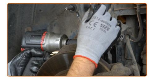
Unscrew the lower fastener connecting the shock strut to the steering knuckle. Use a combination spanner #21. Use a drive socket #21. Use a tap wrench.
