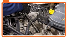
Remove the spark plugs with a spark plug wrench and place them on a work surface in the order of installing in the engine.
