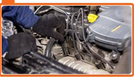
Connect the high voltage wires to the spark plugs.
