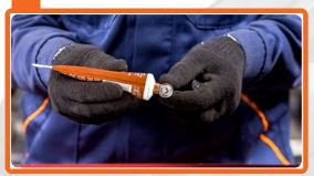
Apply a thin layer of special grease on the thread surface of new spark plugs.
