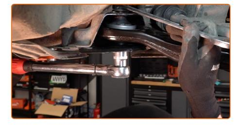
Tighten the rear fastener of the control arm. Use a combination spanner #19. Use a drive socket #22. Use a torque wrench. Tighten it to 95 nm torque.
