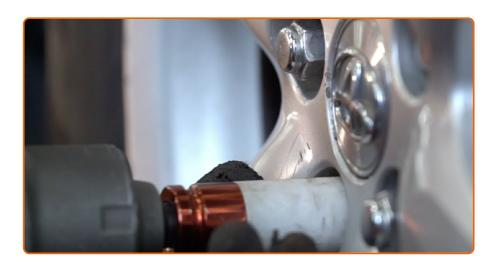
Screw in the wheel bolts. Use wheel impact socket #21.
