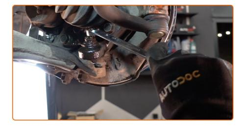
Loosen the fastener connecting the ball joint to the steering knuckle. Use a combination spanner #19.
