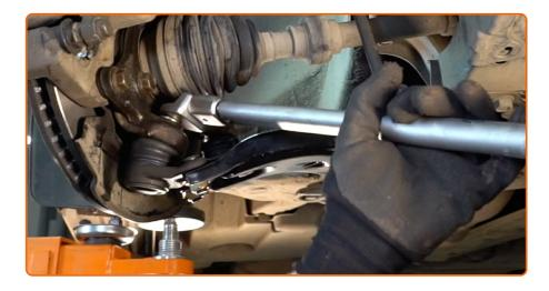
Screw the fastener connecting the ball joint to the steering knuckle. Use a combination spanner #19. Use a torque wrench. Tighten it to 60 Nm torque.
