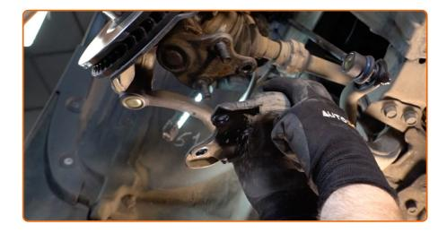
Disconnect the spherical joint from the arm.
