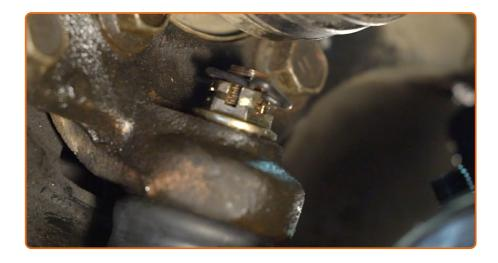
Install the cotter pin. Use round-nose pliers.
