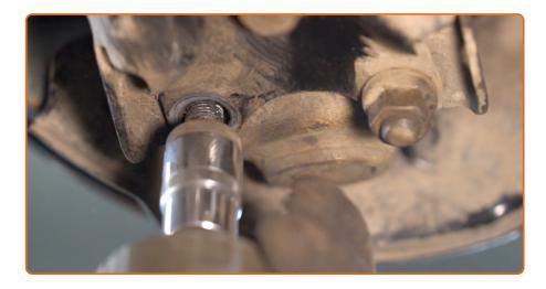
Unscrew the fastener connecting the ball joint to the suspension control arm. Use a drive socket #17.
