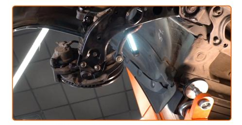
Remove the support from under the arm.
