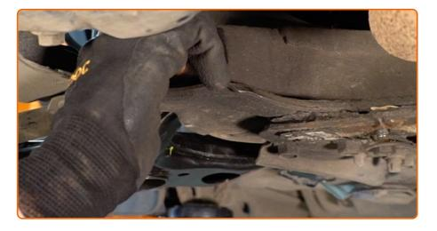
Install the front fastener of the arm.
