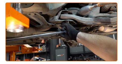
Unscrew the rear arm fastener. Use a drive socket #22. Use a tap wrench.
