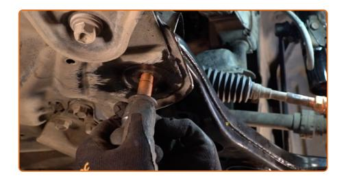
Install the rear fastener of the arm.
