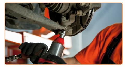
Unscrew the fastener connecting the ball joint to the suspension control arm. Use a drive socket #17. Use a ratchet wrench.
