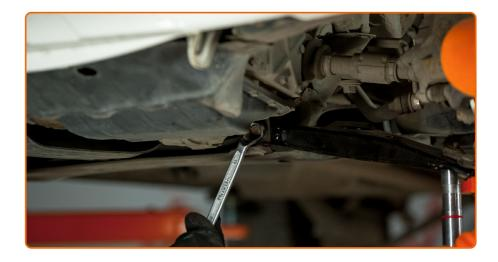
Tighten the rear fastener connecting the arm to the body subframe. Use a combination spanner #19. Use a drive socket #19. Use a torque wrench. Tighten it to 95 nm torque.
