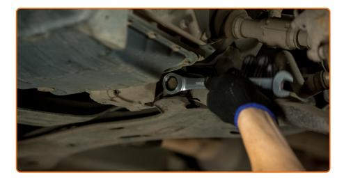
Unscrew the front arm fastener. Use a combination spanner #19.
