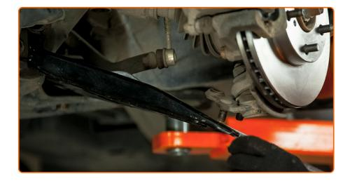
Install the ball joint on the arm and tighten it. Use a drive socket #17. Use a torque wrench. Tighten it to 55 nm torque.
