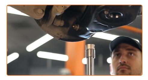
Remove the support from under the arm.
