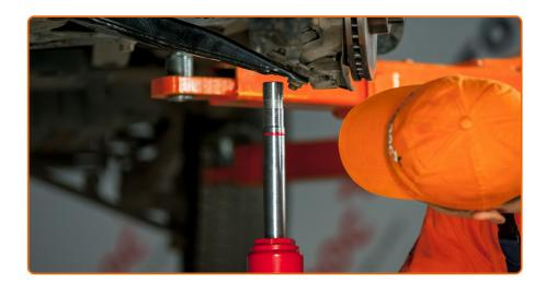
Remove the hydraulic transmission jack.
