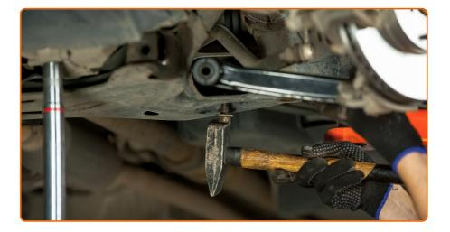
Install the rear fastener of the control arm. Use a crowbar. Use a hammer.
