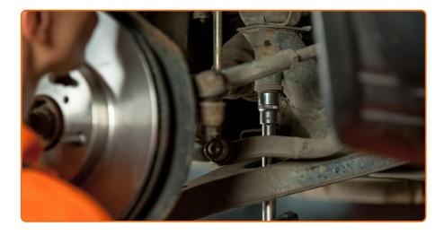
Unscrew the rear fastener connecting the control arm to the subframe. Use a drive socket #19. Use a ratchet wrench.
