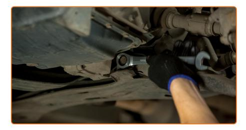
Tighten the subframe fastening. Use a drive socket #19. Use a torque wrench. Tighten it to 95 nm torque.
