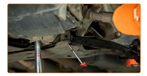
Install a new arm. Use a flat screwdriver.
