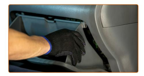
Install the cabin air filter housing. Make sure you hear a click indicating that it is locked in place.
