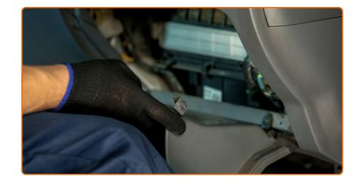
Remove the cabin air filter housing.
