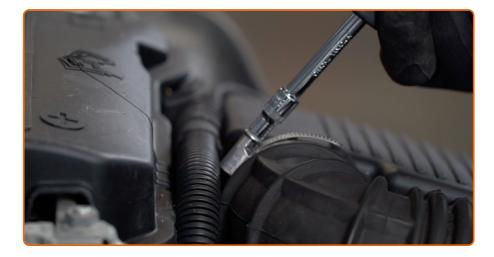
Loosen the clamp and remove the intake air hose from the filter housing. Use a drive socket #6. Use a ratchet wrench.
