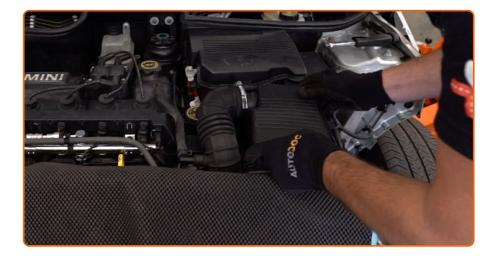
Reinstall the air filter cover. Fasten it.
