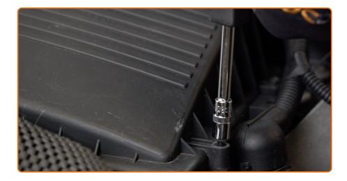
Undo the fastening screws of the air filter cover. Use a drive socket #8. Use a ratchet wrench.
