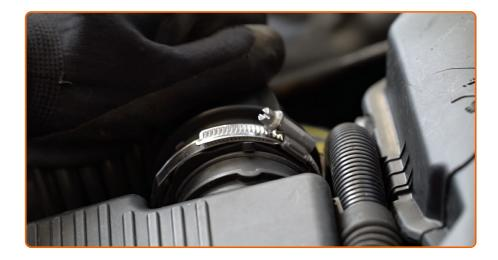
Attach the air intake hose to the air filter housing. Tighten the fuel filter pipe clamp. Use a drive socket #6.
