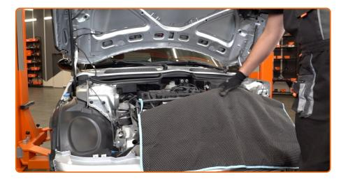
Remove the fender protection cover.
