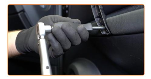
Tighten the door handle fastener. Use a drive socket #10. Use a torque wrench. Tighten it to 15 nm torque.
