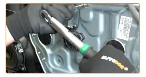
Tighten the door panel fasteners. Use a drive socket #10. Use a torque wrench. Tighten it to 17 nm torque.
