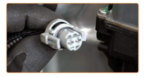
Detach the power window connector. Use round-nose pliers.
