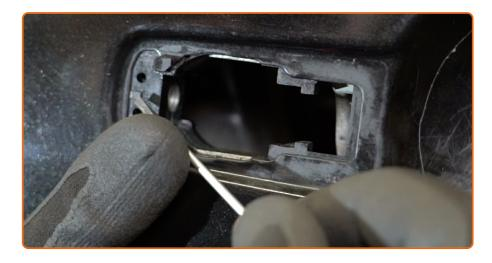
Release the exterior door handle actuator. Use a flat screwdriver.
