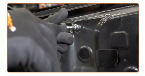
Unscrew the door panel fasteners. Use a drive socket #10. Use a ratchet wrench.
