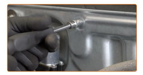
Screw in the door panel fasteners. Use a drive socket #10. Use a ratchet wrench.
