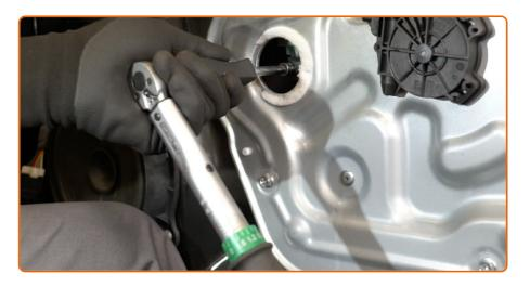
Tighten the window glass fasteners. Use a drive socket #10. Use a torque wrench. Tighten it to 13 nm torque.
