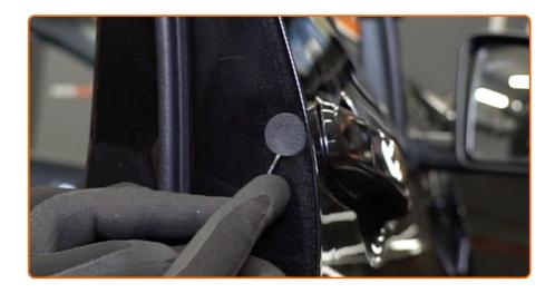
Remove the cover from the exterior door handle fastener. Use a flat screwdriver.
