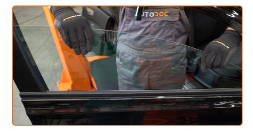
Lower the window glass and install it to its mounting seat in the window raiser mechanism.
