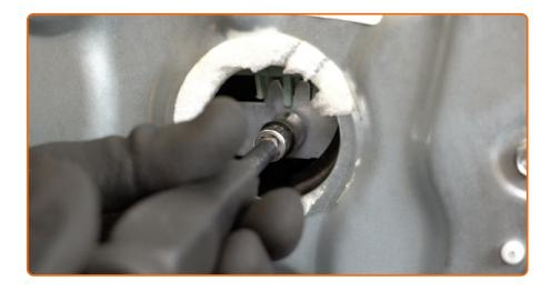
Unscrew the window glass fasteners. Use a drive socket #10. Use a ratchet wrench.
