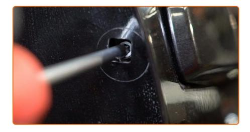
Unscrew the fastener of the exterior door handle. Use Torx T20. Use a ratchet wrench.
