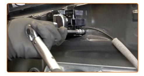
Screw in the interior door handle fastener. Use a drive socket #10. Use a torque wrench. Tighten it to 15 nm torque.
