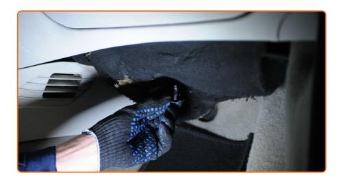
Unscrew the fasteners of the cabin filter housing cover.
