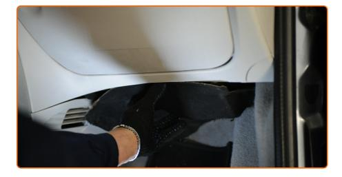
Install the glove box lining and screw in its fasteners.
