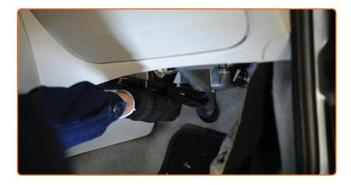
Screw in the fasteners of the cabin filter housing cover.
