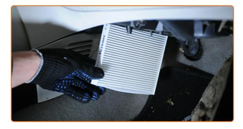
Install the cabin filter to its mounting seat.
