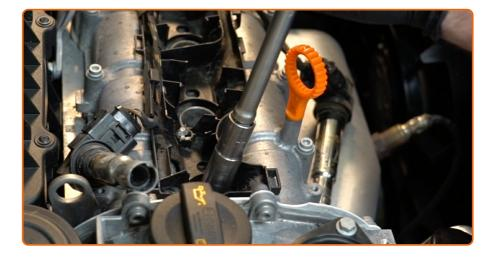
Unscrew the spark plugs. Use the spark plug socket #16. Use a ratchet wrench.
