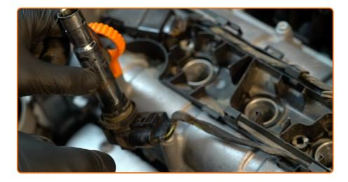
Take out the ignition coils from the spark plug wells. Use a crowbar.
