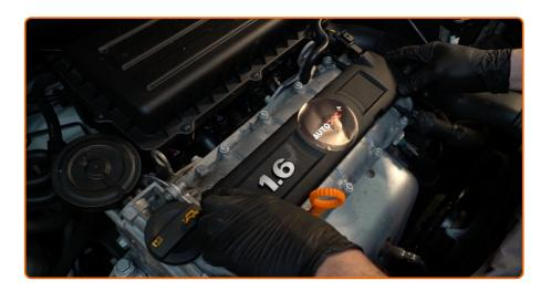
Install the engine cover and secure it.
