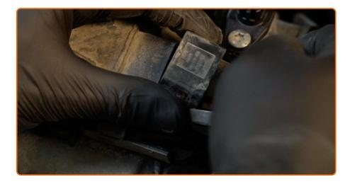
Detach the connector from the ignition coil.
