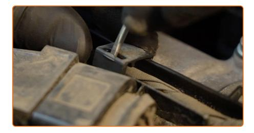
Undo the plastic locking tabs of the ignition coil connector. Use a flat screwdriver.
