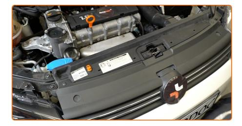
Remove the fender protection cover.
