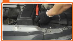
Reinstall the air filter cover. Fasten it.
