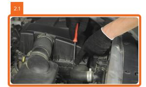
Loosen and remove the air filter cover.
