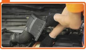
Remove the air filter and replace it with a new one.
