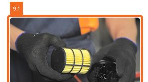
Install a new filter element into the holder, and then the entire assembly into the case, aligning the element upper part with the housing.
