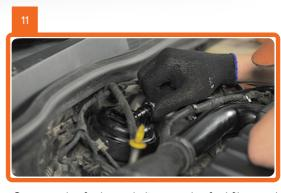
Connect the fuel supply lines to the fuel filter and tighten the fasteners.
