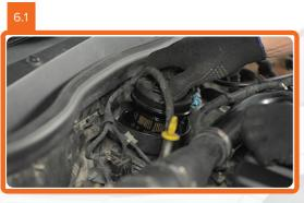
Remove the filter element from the filter housing
