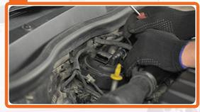
Loosen the fuel supply lines fastening to the fuel filter.
