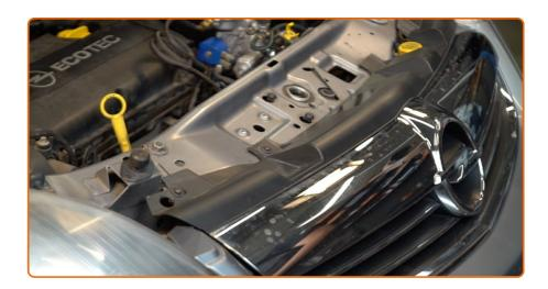
Remove the fender protection cover.
