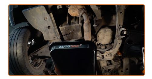
Put a waste oil container with at least 4 I capacity under the drainage hole.
