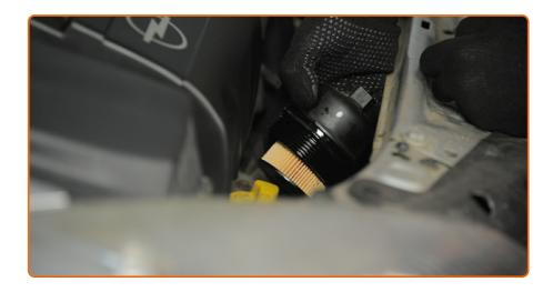
Install a new oil filter housing cover and tighten it.
