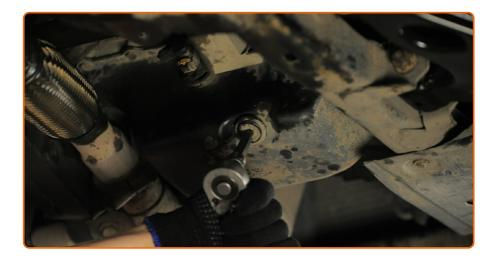
Unscrew the drain plug. Use Torx T45. Use a ratchet wrench.
