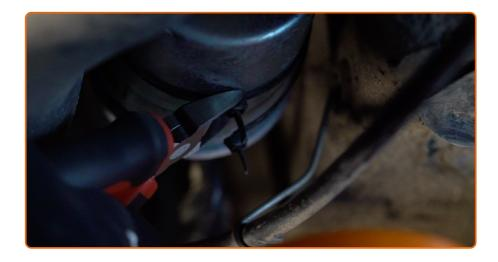
Detach the fuel filter fasteners. Use nippers.
