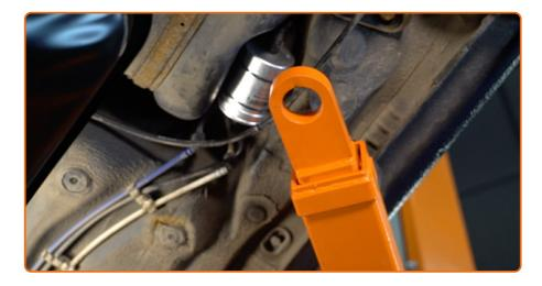
Take the fluid container away from under the fuel filter.
