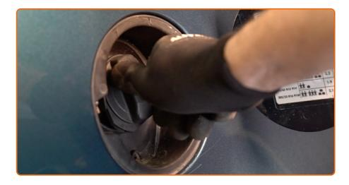
Tighten the fuel filler cap.
