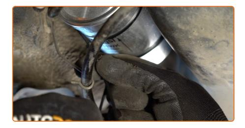
Attach the fuel filter fasteners. Use nippers.
