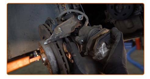
Remove the brake pads. Use a crowbar.
