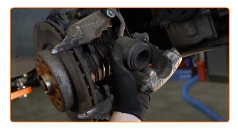
Remove the brake caliper.
