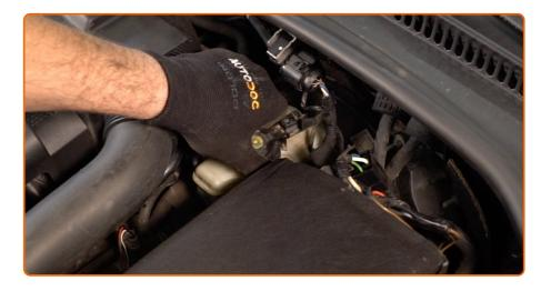
Tighten the brake fluid reservoir cap.
