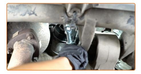
Unscrew the oil filter. Use the 76-F14 socket. Use a ratchet wrench.
