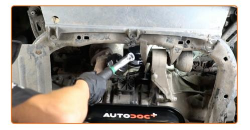
Tighten the oil filter. Remember to observe the recommended tightening torque. Use the 76-F14 socket. Use a torque wrench. Tighten it to 18 Nm torque.
