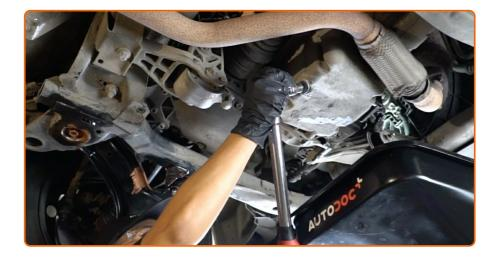
Screw in the new drainage plug and tighten it. Use Torx T40. Use a torque wrench. Tighten it to 24 Nm torque.
