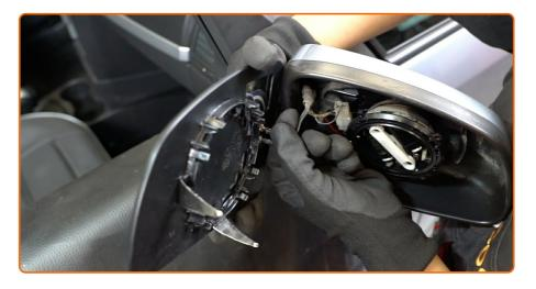
Attach the mirror heating connectors.
