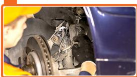
Disconnect the brake hose holder from the shock absorber strut.
