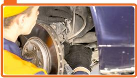
Disconnect the cable fastener of the brake pads wear sensor from the shock absorber strut.
