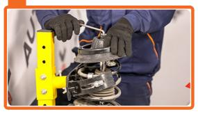
Tighten the upper fastener of the shock absorber strut mount.
