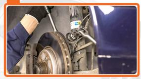
Unscrew the lower fastener of the shock absorber strut.
