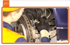
Connect the fastener of the ABS sensor cable to the shock absorber strut.
