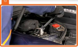
Unscrew the upper fastening of the shock absorber strut.
