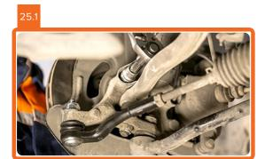
Install the steering knuckle onto the shock absorber strut.
