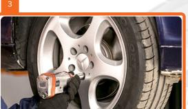
Loosen the wheel mounting bolts.
