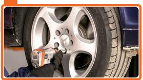
Lower the car and working in a cross order, tighten the wheel bolts
