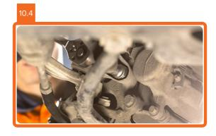
Disconnect the steering knuckle from the shock absorber strut.
