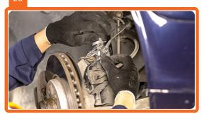
Connect the cable fastener of the brake pads wear sensor to the shock absorber strut.
