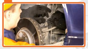
Disconnect the fastener of the ABS sensor cable from the shock absorber strut.
