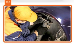
Remove the suspension strut.
