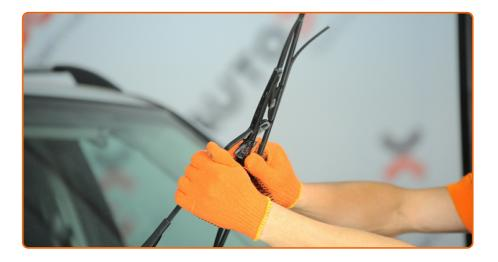
Remove the blade from the wiper arm.
