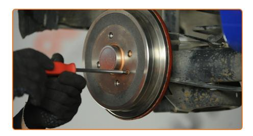
Tigten the brake drum fasteners. Use a Phillips screwdriver. Use a torque wrench. Tighten it to 17 Nm torque.
