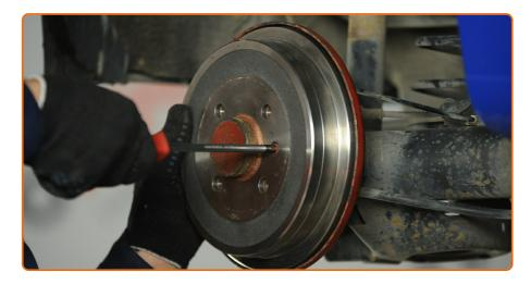
Unscrew the brake drum fastening. Use a Phillips screwdriver.
