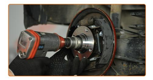
Tighten the hub. Use a drive socket #30. Use a torque wrench. Tighten it to 185 Nm torque.
