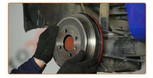
Remove the brake drum.
