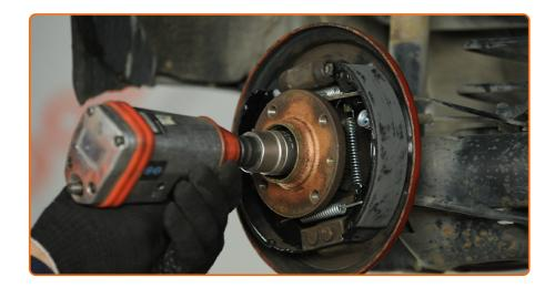
Unscrew the wheel hub axle nut. Use a drive socket #30. Use a ratchet wrench.
