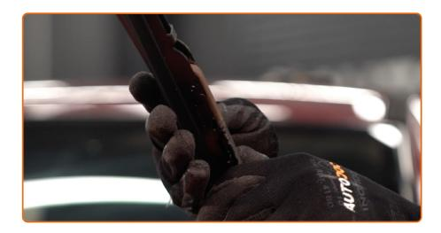
Install the new wiper blade and carefully press the wiper arm down to the glass.
