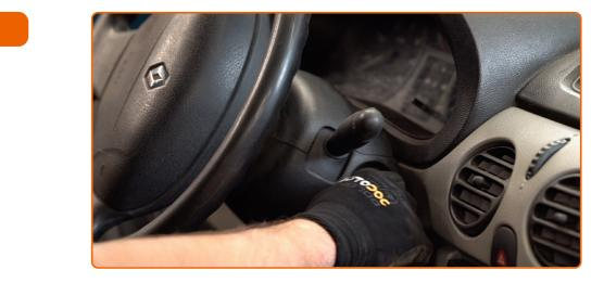
Switch on the ignition. Pull the windscreen wiper stalk to the downward position.
