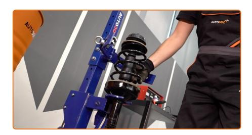
Remove the assembled shock strut.
