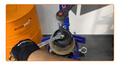
Tighten the shock strut piston rod nut. Use HEX No.H6. Use a combination spanner #14. Use a torque wrench. Tighten it to 55 Nm torque.
