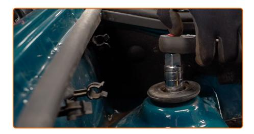
Unscrew the upper fastening of the shock absorber strut. Use a drive socket #21.
