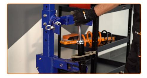
Install the new shock absorber on the hydraulic coil spring compressor.
