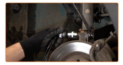
Unscrew the lower fastener connecting the shock strut to the steering knuckle. Use a drive socket #21. Use a combination spanner #21. Use a tap wrench.
