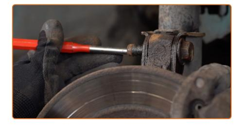
Remove the fastening bolts (2 pieces). Use a hammer. Use a pin punch.
