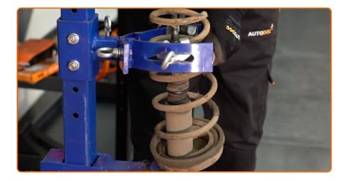
Release the coil spring.
