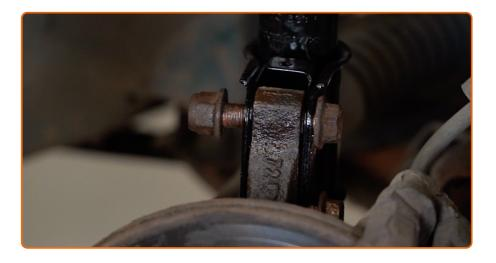
Install and tighten new bolts of the steering knuckle. Use a drive socket #21. Use a combination spanner #21. Use a torque wrench. Tighten it to 95 Nm torque.
