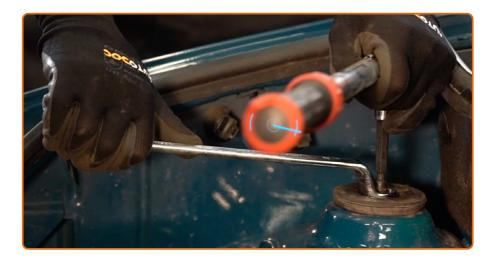
Tighten the shock strut top mount. Use a combination spanner #21. Use HEX No.H6. Use a torque wrench. Tighten it to 30 Nm torque.
