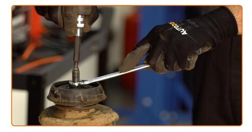
Remove the strut piston rod nut. Use HEX No.H6. Use a combination spanner #14. Use a ratchet wrench.
