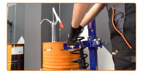
Install the spring on the shock absorber.
