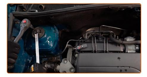
Loosen the upper fastener of the shock strut mount. Use a combination spanner #21. Use HEX No.H6. Use a ratchet wrench.
