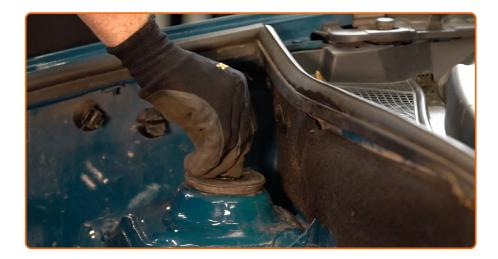
Install the shock strut mount cap.
