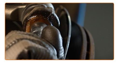
Tighten the fastening nut connecting the tie rod end to the steering knuckle. Use a drive socket #17. Use a torque wrench. Tighten it to 70 nm torque.
