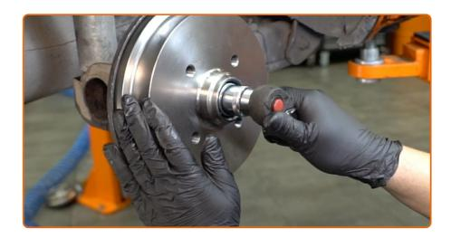
Screw on the hub nut. Use a drive socket #30. Use a ratchet wrench.
