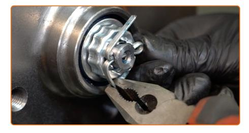
Install a new hub nut cotter pin. Use pliers. Use a hammer.
