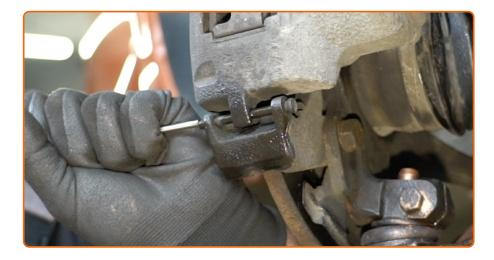
Remove the brake caliper cotter pin. Use a pin punch. Use a hammer.
