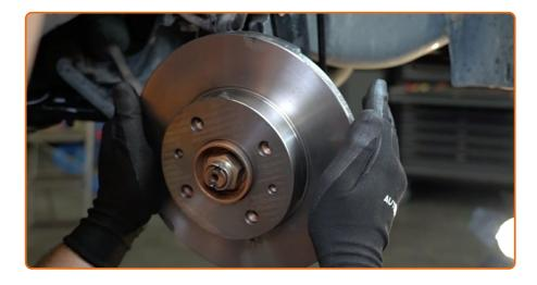
Install the brake disc.
