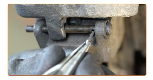
Install the lock pin retainer clip. Use round-nose pliers.
