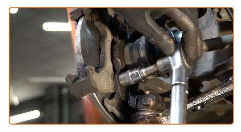
Tighten the brake caliper bracket. Use a drive socket #18. Use a torque wrench. Tighten it to 70 Nm torque.
