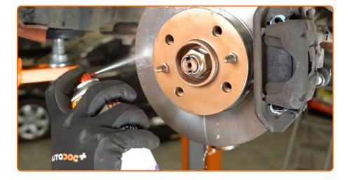
Treat the surface where the brake disc contacts the wheel rim. Use copper grease. Clean the brake disk surface. Use a brake cleaner.
