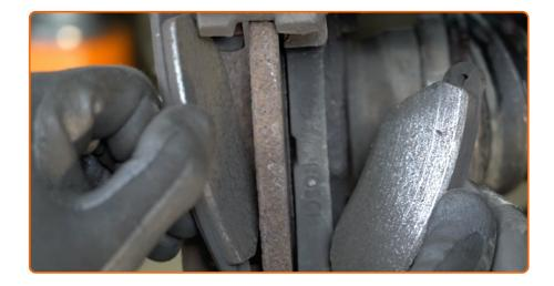
Remove the brake pads.
