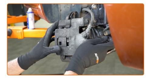
Install the brake caliper and fix it.
