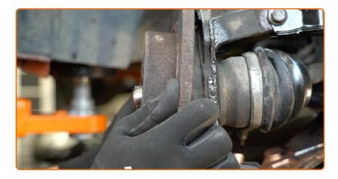
Remove the brake disc. Use a rubber mallet.
