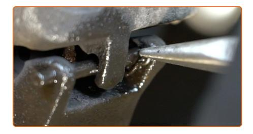
Remove the lock pin retainer clip. Use round-nose pliers.
