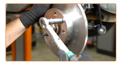
Tighten the brake disc fastening. Use a drive socket #12. Use a torque wrench. Tighten it to 8 Nm torque.
