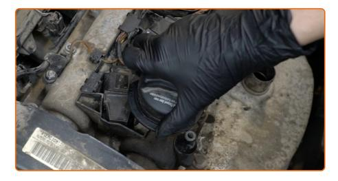
Install the oil filler neck. Screw in the oil filler neck.
