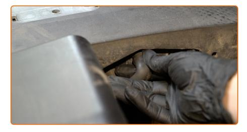
On the right side, attach the PCV valve hose to the engine cover.
