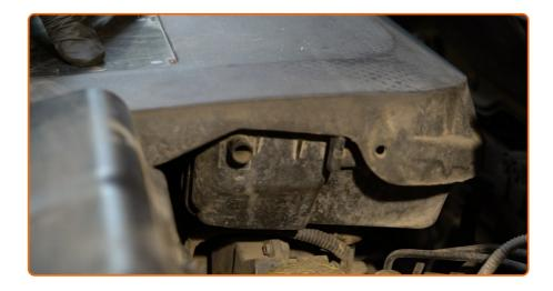
Install the engine cover and secure it.
