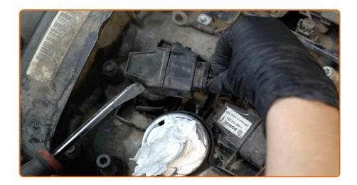
Take out the ignition coil from the spark plug well. Use a crowbar.
