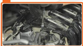
Tighten the ignition coil fastening.
