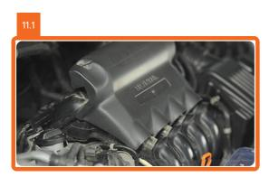
Install the engine cover and secure it.
