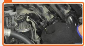
Connect the plugs to the ignition coil.
