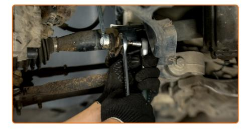
Unscrew the fastener connecting the stabilizer link to the stabilizer bar. Use a combination spanner #19. Use HEX No.H5. Use a ratchet wrench.
