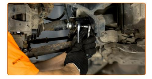
Tighten the fastener connecting the stabilizer link to the stabilizer bar. Use a combination spanner #19. Use HEX No.H5. Use a torque wrench. Tighten it to 60 Nm torque.
