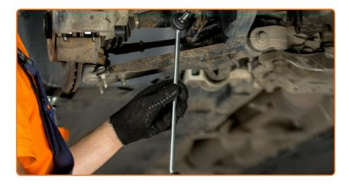
Install a new rod, tighten the fasteners.
