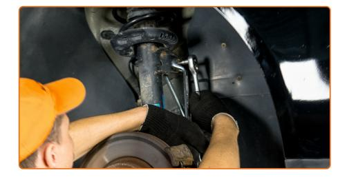
Unscrew the fastener connecting the stabilizer link to the shock strut. Use a combination spanner #19. Use HEX No.H5. Use a ratchet wrench.
