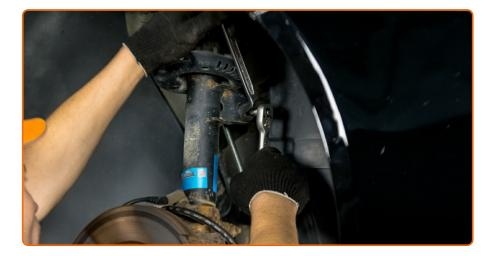
Tighten the fastener connecting the stabilizer link to the shock strut. Use a combination spanner #19. Use HEX No.H5. Use a torque wrench. Tighten it to 60 Nm torque.
